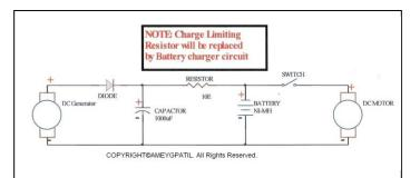
Fig.2 is a schematic diagram of internal circuit of Pico-hydro-electric toothbrush.
